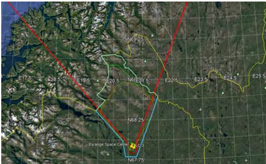
Figure 3-5: From Esrange User’s Handbook Volume IX Spaceport, page 8, showing azimuths between 320° and 020°.
